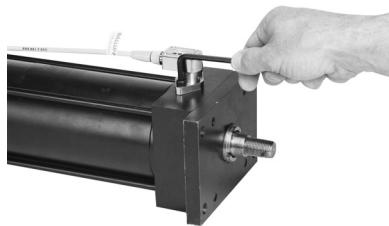
Bolt sensor to cylinder.
